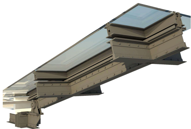
Figure 1. Waterloo Station, an example of parametric variations of a truss system. While these two assemblies look different, they can be seen as two parametric variations of a single design.
