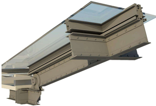
Figure 2. Parametric variations of the roof/skylight assembly (BIM model).
